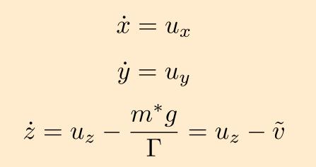
Where  $u_i$  is the fluctuating velocity
